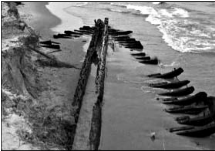
Keel, floors and ribs of the 1882 wrecked schooner Comet.
