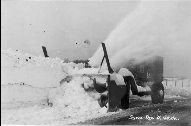
A Sno-Go snowblower machine is tackling a big snowdrift on an Oceana County road.
