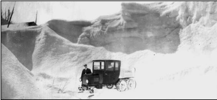
A Sno-Go snowblower machine is tackling a big snowdrift on an Oceana County road.
